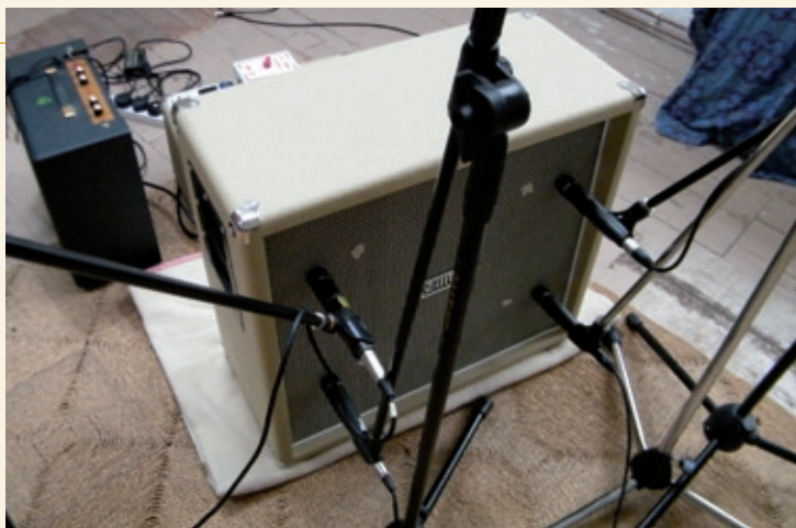
The four miking configurations used to record our audio examples.
