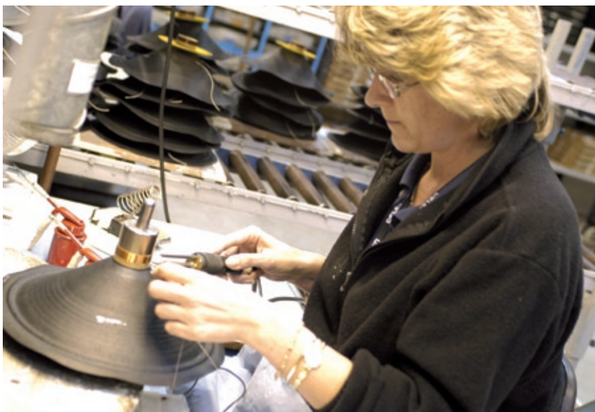
A loudspeaker is born in the Celestion factory. Here, the cone assembly is being constructed.
