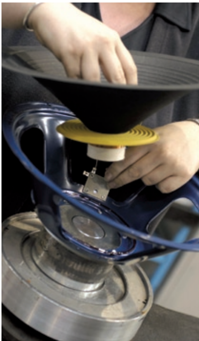
The completed cone assembly being inserted into the speaker frame.
